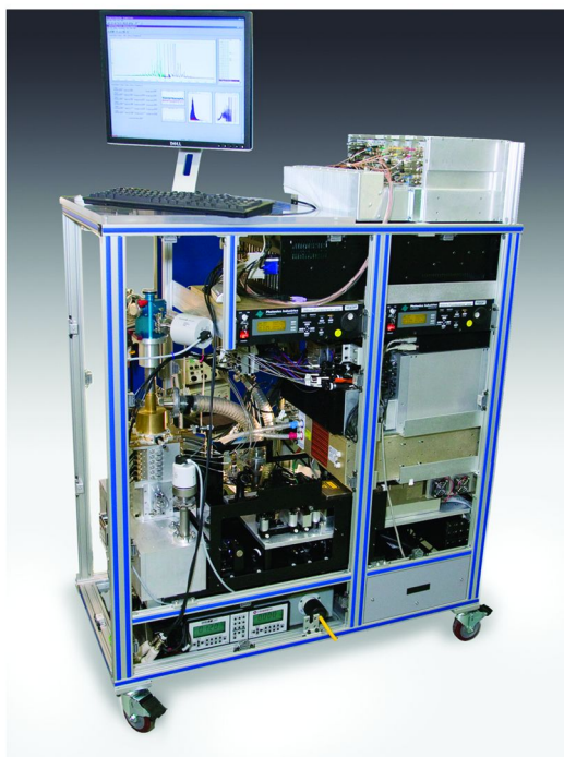
Figure 1. (a) Photo of the SPAMS system prototype (SPAMS 1.3) used to produce most of the results described here. A second generation SPAMS system (SPAMS 2.0, shown in (b)) was built for a DoD sponsor and is only half the size of the system shown (a). Even smaller SPAMS instruments are currently under development by Livermore Instruments Inc.
